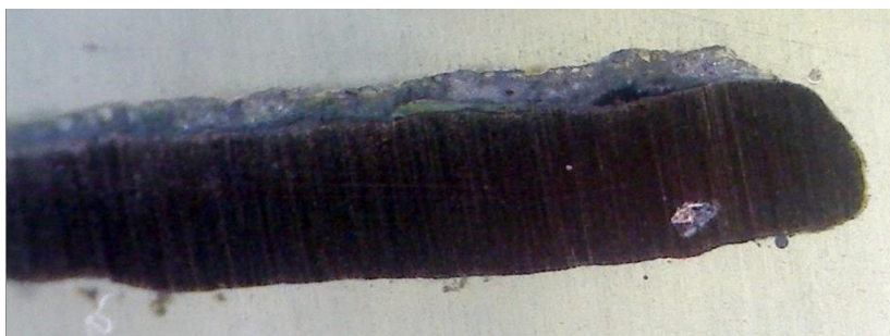
Fig. 5 Macrostructure of the coin metal (Id 10) (25× magnification) showing a non-deformed slag inclusion in the right section of the coin's cross-section
